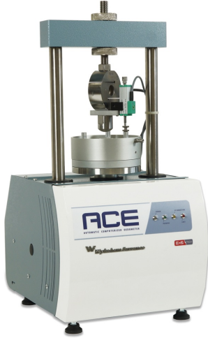
ACE EmS - Electromechanical Servoactuation, automatic oedometer machine (26-WF31E20) complete with consolidation cell (26-WF0320)
